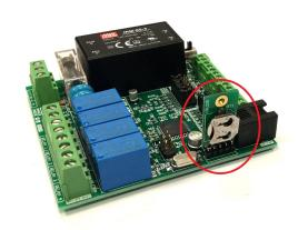
You must activate the pull-up resistors on the I2C bus for the correct operation of the RTC.
